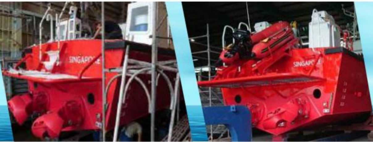
RFV1G (left) vs RFV2G on the right, which is equipped with an IRB (Inflatable Rescue Boat) for deployment in shallow water operations
