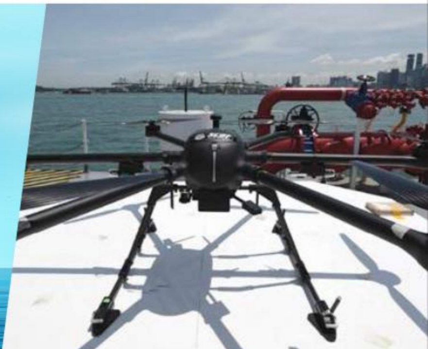
Gimbal-stabilized platform compensates movement and allows deployment of UAV while vessel is making way
