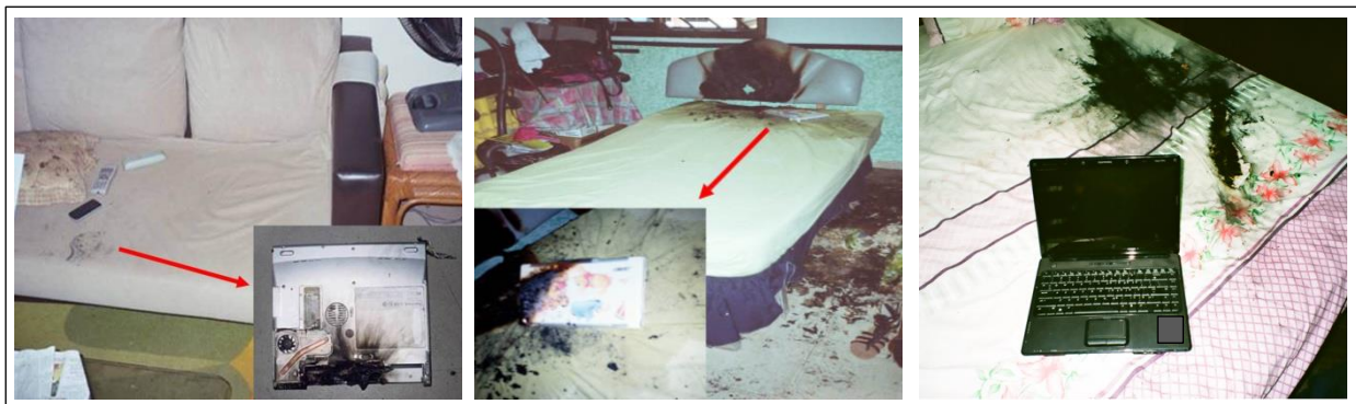
Figure 14. Laptop battery fires occurred on the bed or sofa
