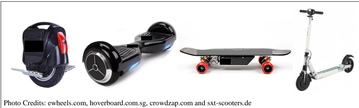
Figure 7. Personal Mobility Devices (left to right): e-wheel, hoverboard, electric skateboard and electric scooter
