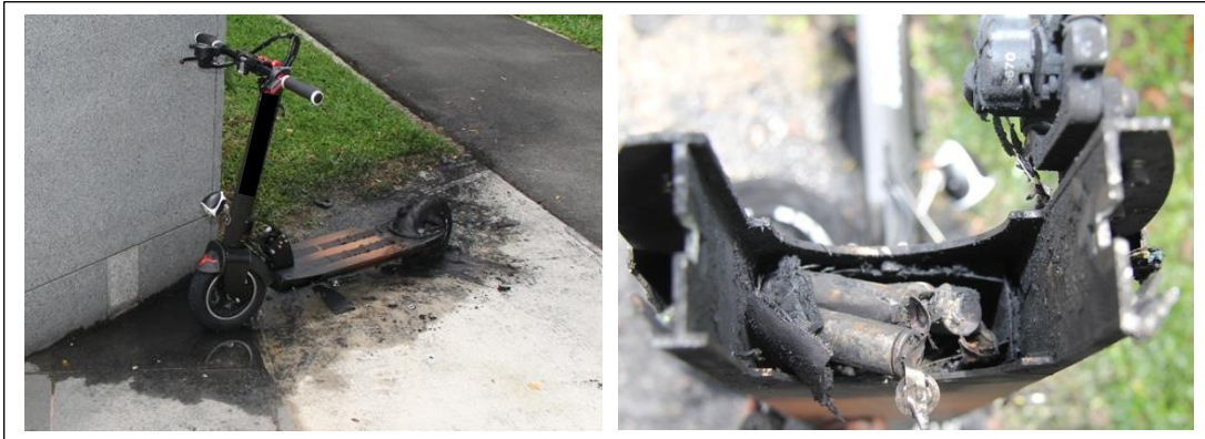
Figure 8. An electric scooter and the batteries affected in the fire
