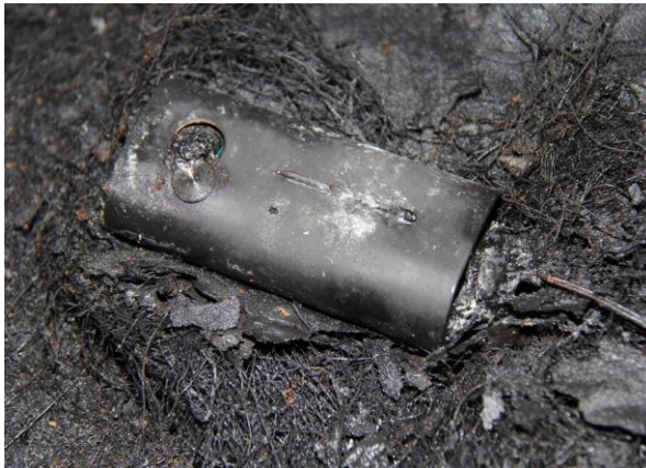
◀ Figure 23. Burnt remains of the powerbank were recovered from the determined Area of Fire Origin
