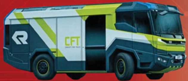
Figure 8: Rosenbauer Concept Fire Truck – electric pump ladder
