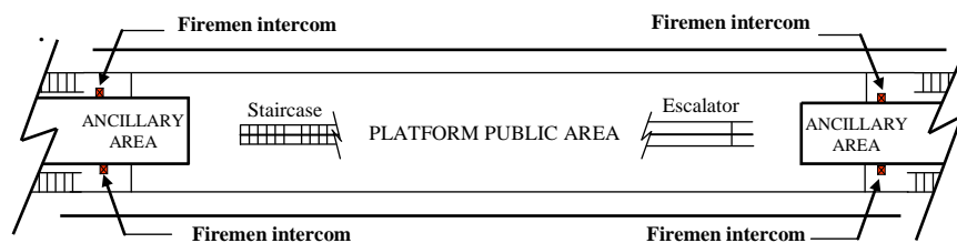
Locations of firemen intercom at platform level
