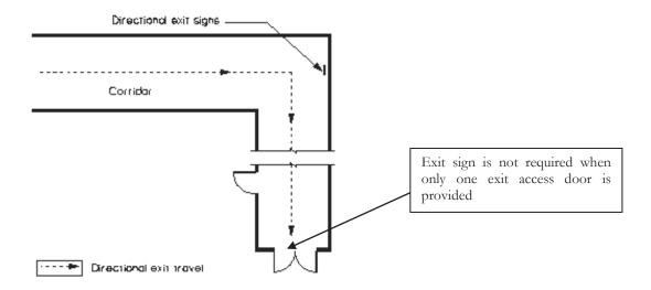
c. <u>In a room provided with emergency lighting</u>, exit sign is not required if there is only one exit access door
