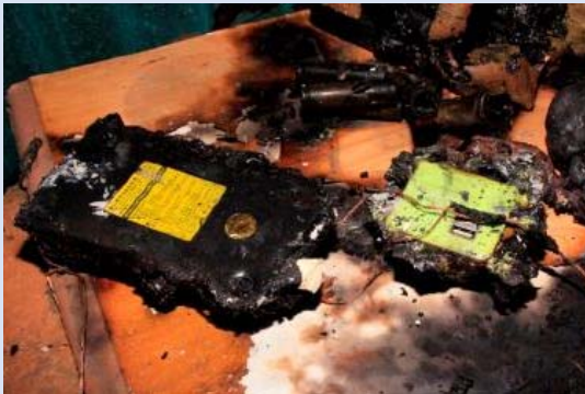
Close up view of the burnt e-bicycle battery
