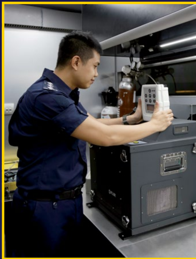
▲ CPT Chin Nam using the Griffin Gas Chromatography-Mass Spectrometry (GCMS) system which has been incorporated into the HCV recently.
