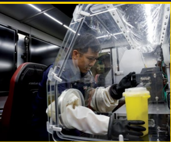
▲ Emergency First Responders can hand over the sample to the DHOs via an opening on the HCV. DHOs will then conduct the required tests on these samples within this box.
