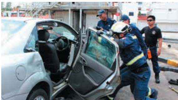
Figure 4– Bend the B Post and two doors downward
