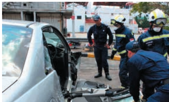
Figure 5 – Fully exposed B-Post makes cutting easy
