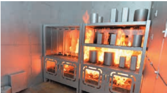
Figure 4: Storage Rack Scene Prop configured on the MFT
