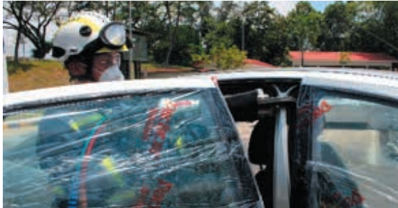
Figure 2 – Cut the top of B Post
