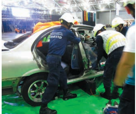
Figure 8 – A participant correctly supporting the B-post to prevent excessive dislodgement
