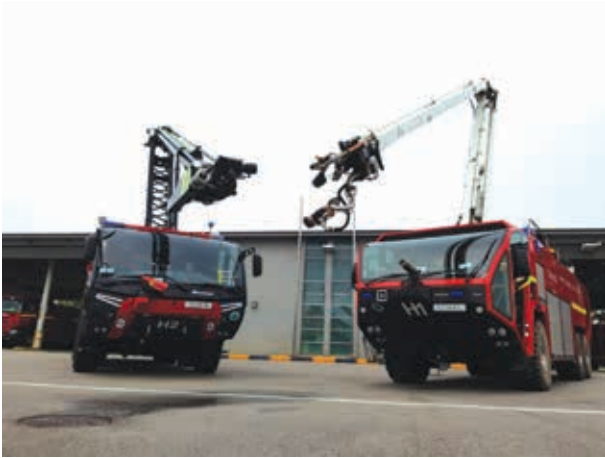
Figure 1: Changi Airport's HRETs poised in action, with the piercing tips deployed. The Rosenbauer "Stinger" is on the left, and the Oshkosh "Snuzzle" is on the right.
