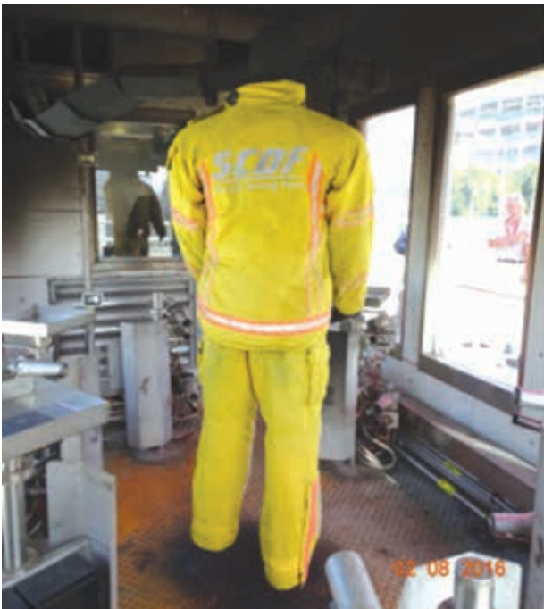
Figure 6: SCDF TOG garment undergoing Thermo-Man™ testing
