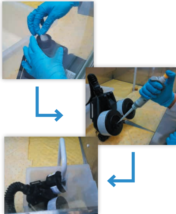
Figure 8: A Tenax mesh was put at the air outlet of the PAPR before the experiment. The filter canisters were then spiked before rinsing under running tap water to simulate wet decon.
