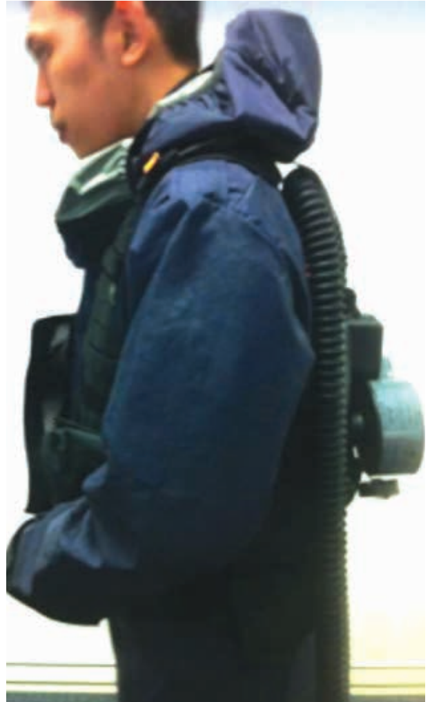
Figure 5: A responder wearing the Saratoga 6-hour Chemical Protective Coverall and the PAPR with canisters mounted on his back
