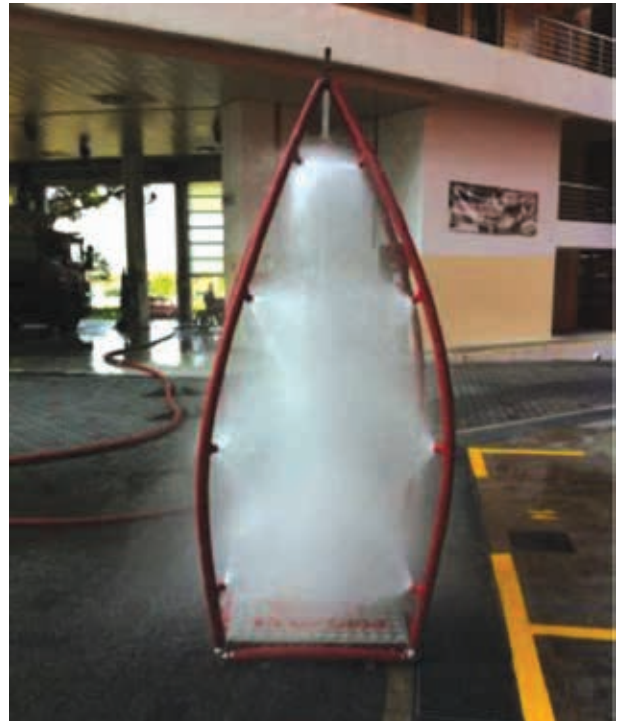
Figure 6: A fully-charged Portaflex shower, forming a frame by the four shower legs
