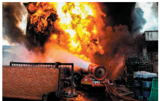
Figure 6: Unmanned Fire Fighting Machine in action
