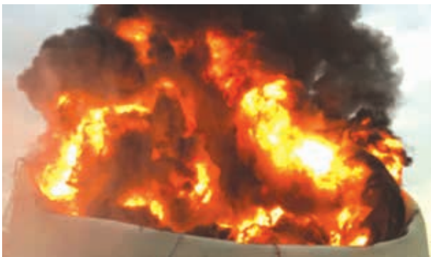
Figure 7: ‘Inward folds’ formed along the rim of the affected tank where it buckled inwards due to the intense heat created persistent pockets of fires where the foam layer had difficulty blanketing.
