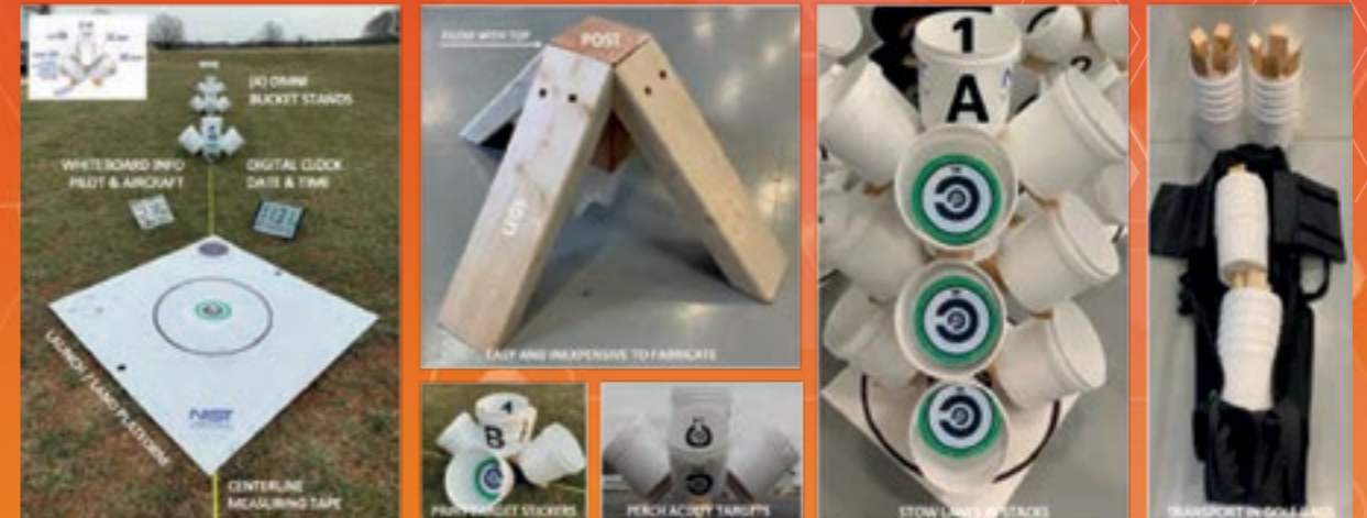
Test apparatus can be easily stored by stacking or, with hinged legs, collapsed into nylon golf club bags which are compliant with airline baggage rules.
