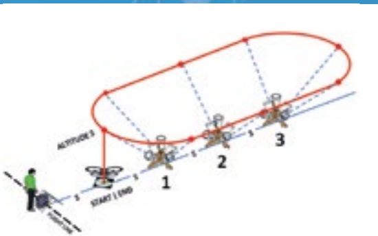
Two transverse flight orbits are completed during the second state of the Basic Proficiency Evaluation for Remote Pilots.
