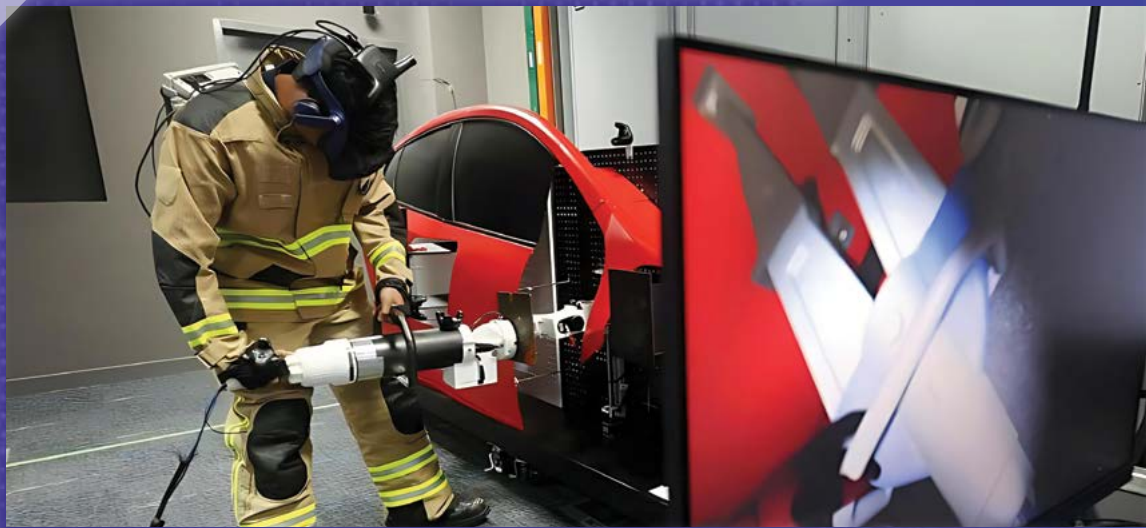
Figure 1. Trainee performing extrication with replicated XR spreader cutter
