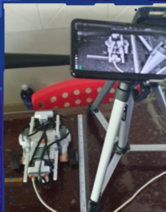
Figure 8: Setup of the second experiment where the robot was programmed to move at different speeds: 1^\circ/\text{sec} , 1^\circ/\text{min} and 1^\circ/\text{hour} .
