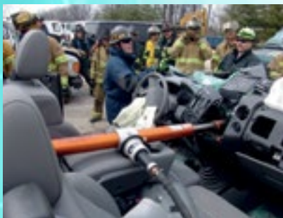
Centre dash ram push evolution on a Ford F-350 Super Duty crew cab pickup truck.
