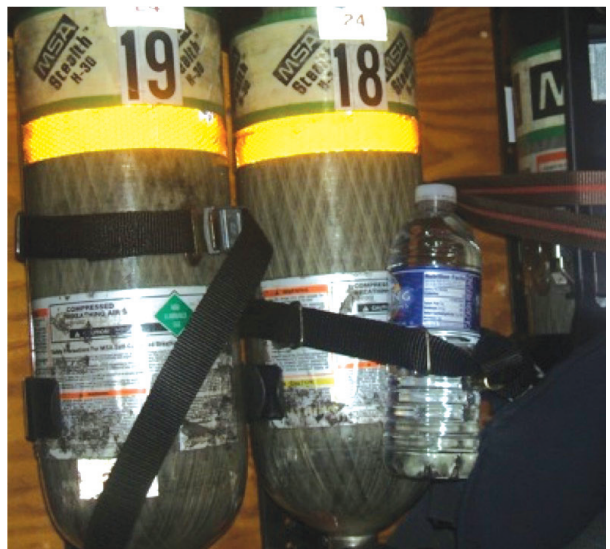
Figure 2: Storing bottled water with spare SCBA cylinders provides immediate access and a visual reminder for the firefighter to rehydrate during an incident.
