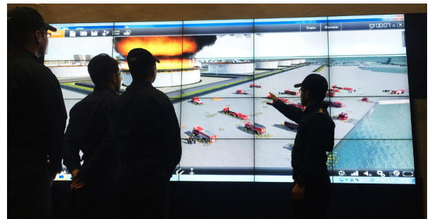
Figure 6: A 4m by 2m large video wall used to conduct briefing and debriefing sessions. With the playback feature, specific instances in the simulation can be shown during debriefs.
