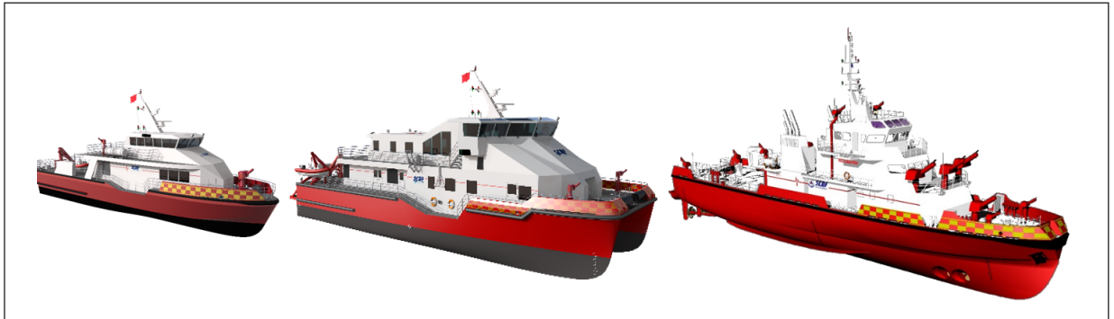
Figure 8: (from left to right) 3-Dimensional Impressions of the Marine Rescue Vessel (MRV), Heavy Rescue Vessel (HRV) and Heavy Fire Vessel (HFV).
