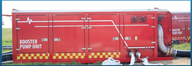
Booster Pump Unit (BPU)
