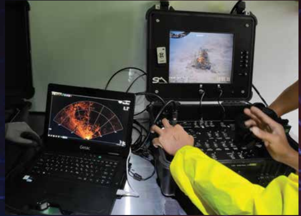
Figure 9: Rescuers operating the ROV with sonar imaging and RGB camera
