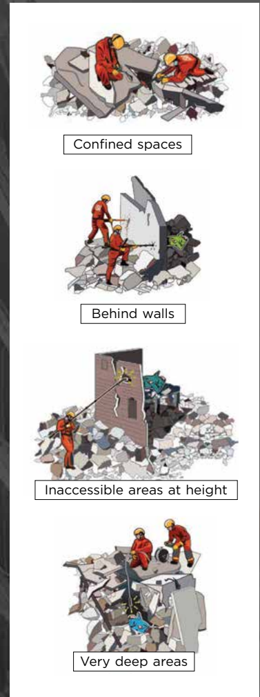
Figure 3: Spaces search cameras allow rescuers to inspect
