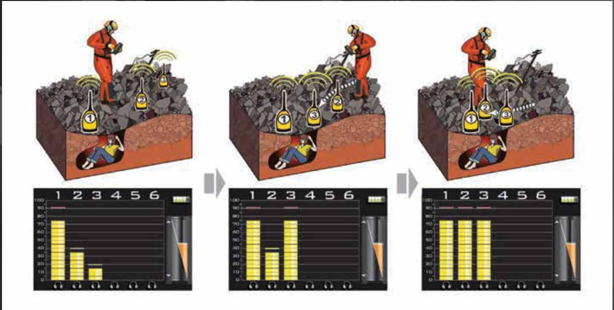
Figure 2: Illustrations of how to use LEADER seismic sensors to find a victim under rubble
