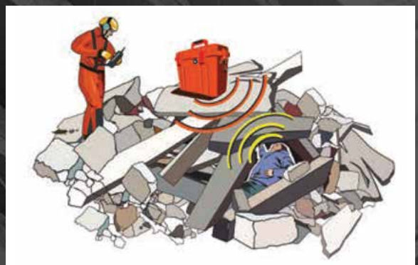
Figure 3: LEADER UWB radar sensor in use on the field
