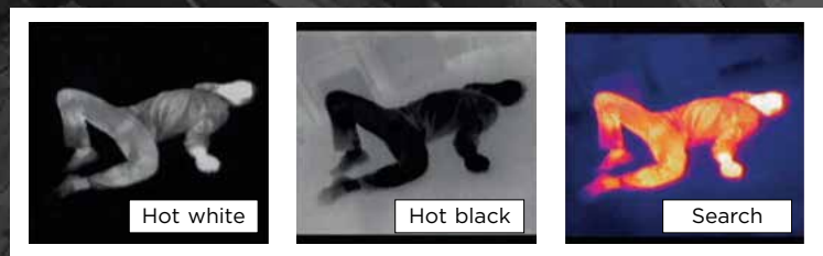
Figure 4: Colour modes of TIC: hot white, hot black and search (multicolour)
